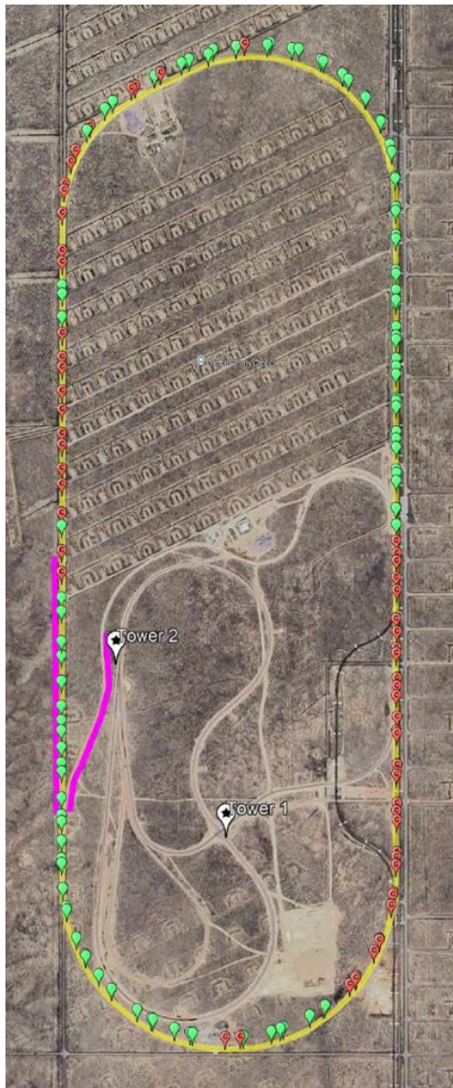
Figure 10-6 Packet loss for HSL7 HOT-to-EOT, 8 repetitions with 10 dB additional attenuation with the train traveling in a clockwise direction.
