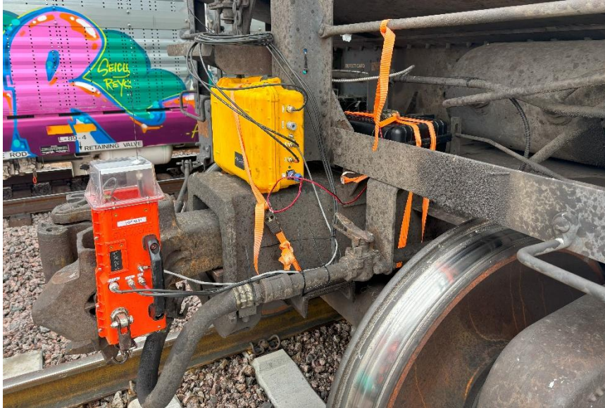
Figure 6-3 Magellan EOT System Installation
